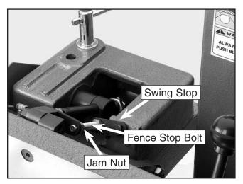
Figure 50. 90° swing stop engaged.
